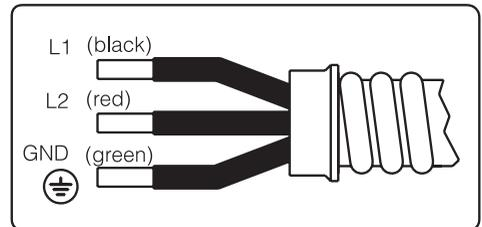
A dedicated line and junction box should be used to connect the cooktop to a 40 A circuit.
